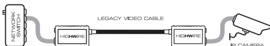
HIGHWIRE units are used to convert conventional Ethernet to a signal that can be carried by 75ohm coaxial video cables such as RG59.
