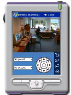
**Tip:** You are also able to control the position of a PTZ camera by using the navigation buttons on the PDA itself.
