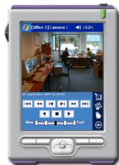
**Tip:** You are also able to use the navigation buttons on the PDA itself for controlling playback: Left button starts reverse playback, right button starts forward playback, center button stops playback,
