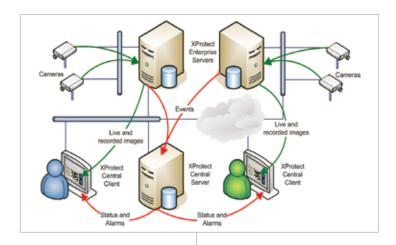
XProtect Central can integrate with security devices such as intruder or access alarms via camera relay inputs or through software integration. The XProtect Central server receives events and status information from the XProtect Enterprise installations and presents it for the operators on the XProtect Central client screens.
