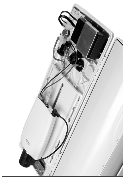
Camera housing with AXIS 211 installed
